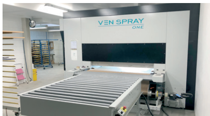
Outfeed of the spray coating machine with subsequent roller conveyor
